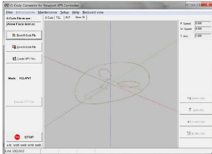
During execution, the stages' encoder position feedbacks are used to draw the actual trajectory executed by the stages.
