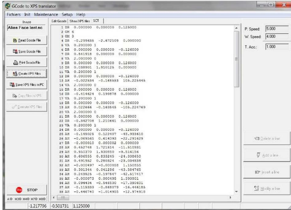
SCT format is a simple way to describe trajectory elements. Each line represents a move or an action.
